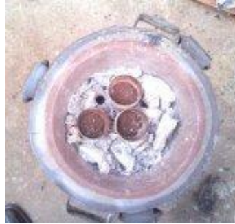
Plate 1. Charcoal Burner with fire clay crucibles containing laterite-charcoal mixture.
